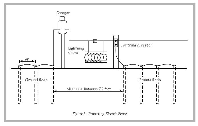
jump the carbon discs inside the lightning arrestor, then disperses the charge to ground. Lightning always finds the quickest and easiest way to earth. Thus, earth/grounding system of the lightning arrestor must be as good as, or better than, the grounding system of the controller. In bad lightning areas, grounding the top wire of the fence has helped protect the controller.
