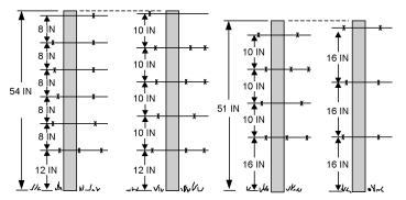
Figure 2. Common wire spacings for barbed wire fences.
