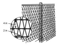
Figure 4. Detail of a diamond-mesh fence.
