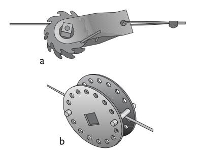
Figure 5a and b. In-line strainers used to tighten and maintain tension are available in two types: a) the ratchet strainer; and (b) the "daisy" strainer. The ratchet strainer requires a special handle for tightening. A 1/2-inch drive ratchet can be used to adjust the "daisy" strainer.
