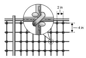
Figure 3. Detail of a square knot-mesh fence.
