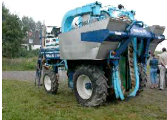
Figure 1: Self propelled Braud 2720 harvester, for black currant harvest. Features pulsating arms, conveyer cups, and 4 aspirators to remove leaves and crop debris. (Value $150,000 new).
