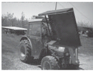
Figure 6. Flamer raised for easy transport and repairs or adjustments.
