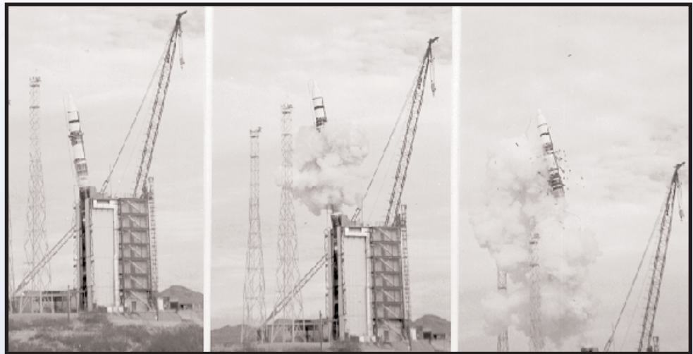
Left, a mock 195,000-pound simulated MX missile, without propellents starts its 300-foot ascent from its launch tower. Middle, the missile continues its ascent. Right, the protective pads begin to fall away, the mock missile will soon start its descent into a large earthen pit about 100 feet downrange.
