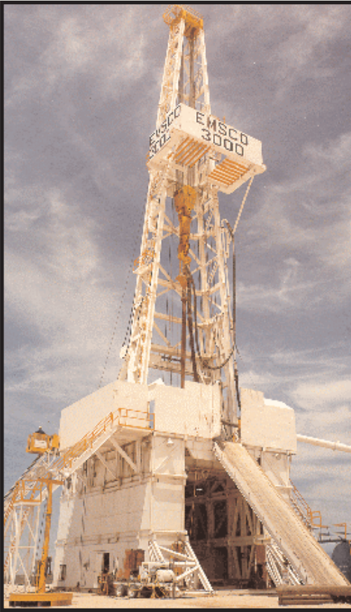
The EMSCO 3000, one of the largest drill rigs used at the Nevada Test Site.
