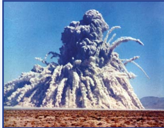
As part of the Plowshare Program, Sedan tested excavation capabilities of nuclear weapons for peaceful purposes.
