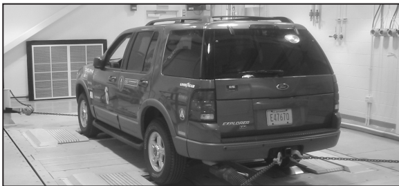
The APRF's 4WD chassis dynamometer can benchmark powertrains for 4WD cars, trucks, and SULEVs.
