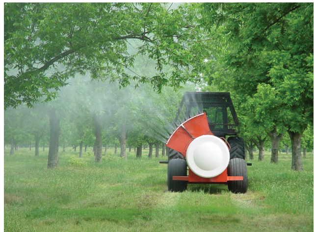
Figure 8. Airblast sprayer used for treating pecan orchards for pecan weevil and other pests.
