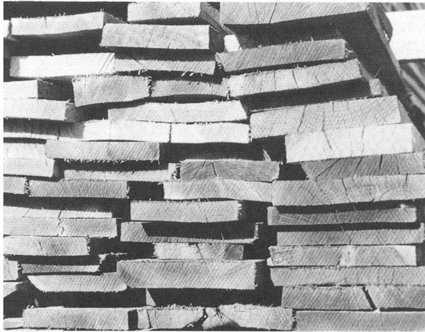
Figure 1. – Excessively thick or thin lumber reflects inefficient mill operation and is a waste of sawtimber resources.
