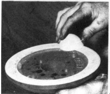
Figure 48. — Test for taper condition of saw collar by the following 3-step process: (A) first chalk the bearing surface. (B) scrape a machined straight-edge across the full face of the collar; if chalk is removed from the outer edge only, taper is all right. (C) if chalk is removed the full width of the bearing surface, taper is lacking.
