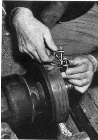
Figure 47.—Check the fast saw collar for trueness with a dial test indicator. A collar that deviates by more than .002 to .003 inch per revolution needs to be remachined.
