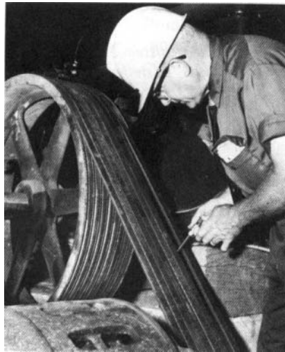
Figure 43. – Check for proper belt tension with a V-belt tension tester.
