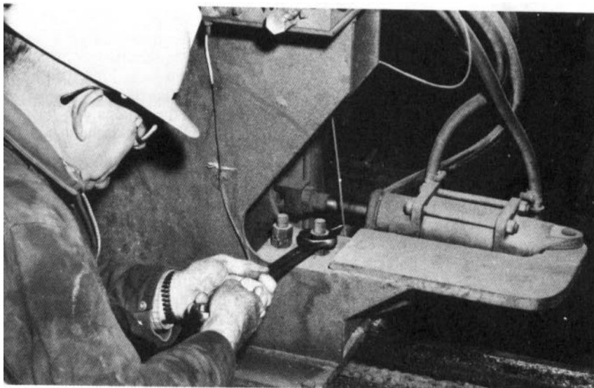
Figure 51. – Most carriages make provision for adjusting knee alignment. On this carriage with chain driven knees, knee alignment is changed by loosening one of these nuts and tightening the other.
