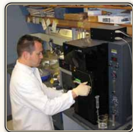
Adam Stoklosa, PhD student, loading a sample into a gravimetric moisture sorption balance to gather information on water-solid interactions.
