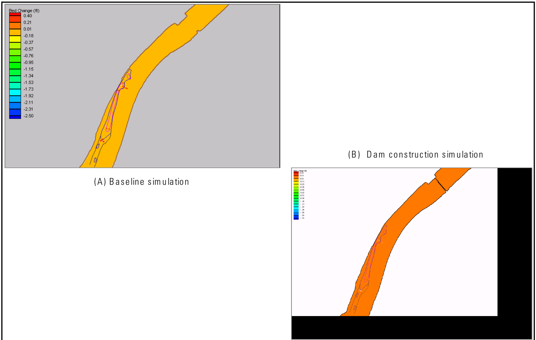
Figure 27. Bed change during low-flow conditions (1997 hydrograph, step 7) for (A) baseline simulation and (B) phase 3 of the Olmsted construction in the study reach near Olmsted, Illinois.
