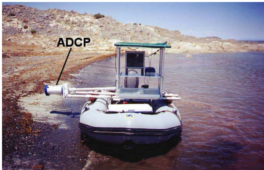
Figure 2. Acoustic Doppler current profiler (ADCP) mounted to an inflatable boat.
