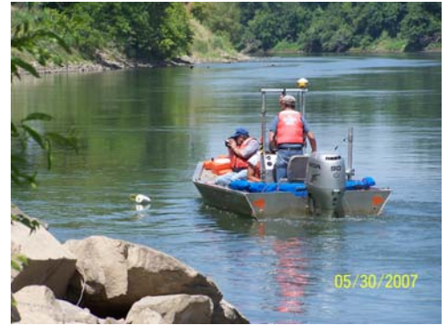
Figure 4: ADCP testing: Range finder used to determine edge estimate. "End-of-transect" marker buoys also deployed for use.
