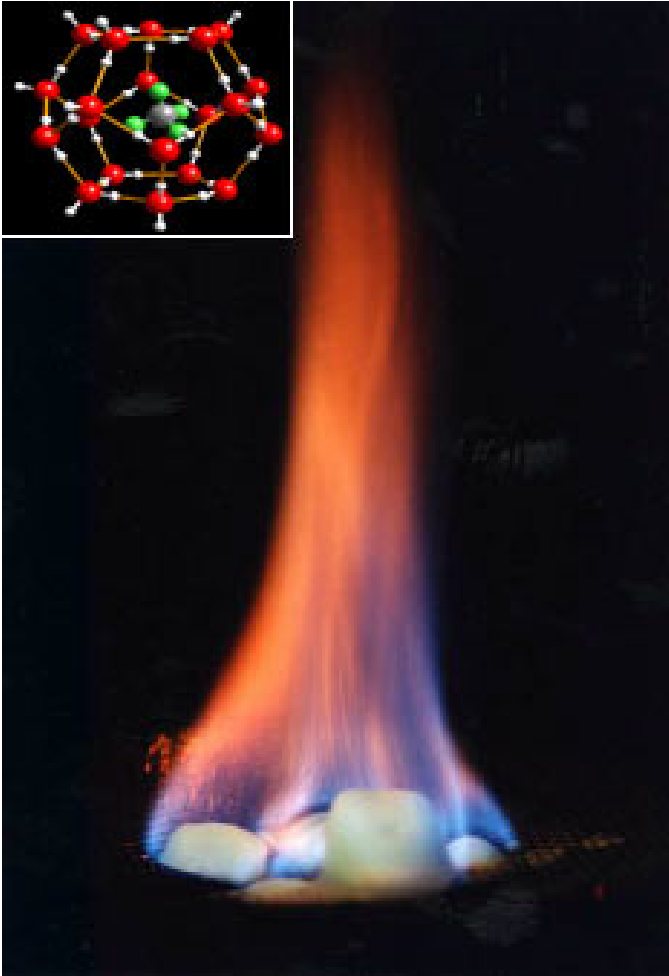
Figure 1.9. A piece of methane clathrate displays its potential as an energy source. As the compound melts, released gas feeds the flame and the ice framework drips off as liquid water. Inlay shows the clathrate structure. Source: U.S. Geological Survey.
