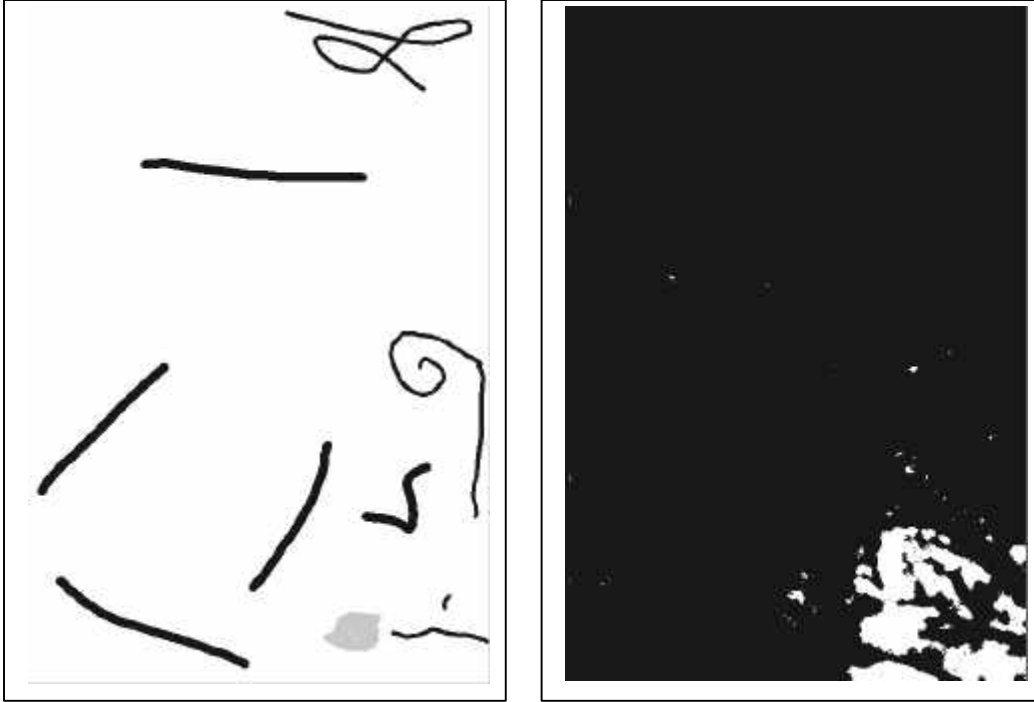
Figure 2. Town/Urban feature. Left: Training data provided to GENIE. Black pixels define non-town training example pixels, and gray pixels define town example pixels. Right: The GENIE result. Town/Urban was detected in pixels marked in white. Compared to the training data (i.e., only those pixels given a true or false label in left panel), this result achieved a detection rate of 100% and a false alarm rate of 0.16%. Outside of the training pixels, performance is qualitatively good, based on comparison to existing, manual land cover maps and known town boundaries.
