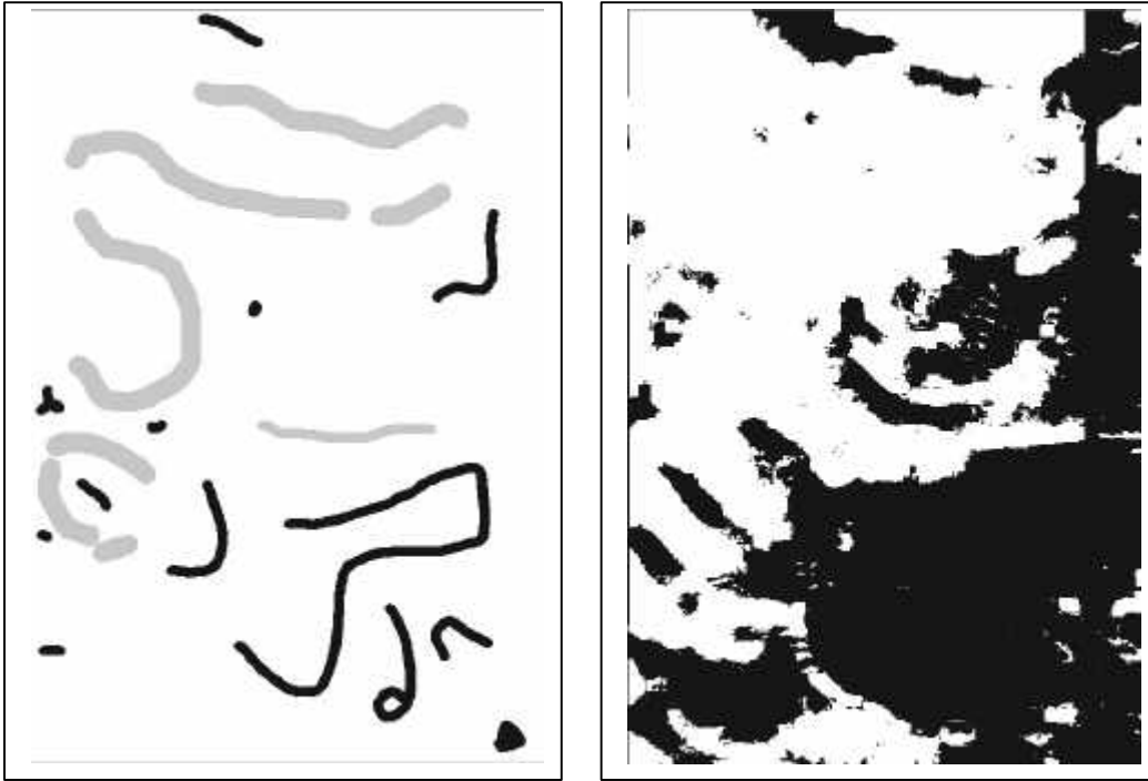
Figure 3. Generic forest feature. Left: Training data provided to GENIE. Black pixels define non-forest training example pixels, and gray pixels define forest example pixels. Right: The GENIE result. Forest was detected in pixels marked in white. Compared to the training data, this result achieved a detection rate of 99.4% and a false alarm rate of 0.5%. Outside of the training pixels, performance is qualitatively good, based on comparison to existing, manual land cover maps.
