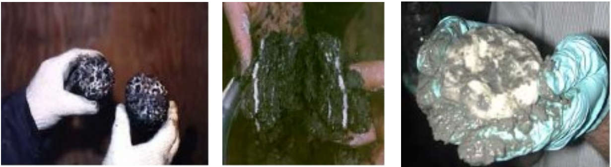
16 Figure 5.3. Photographs of methane hydrate as nodules, veins, and laminae in sediment. 17 Courtesy of USGS 18 ( http://geology.usgs.gov/connections/mms/joint_projects/methane.htm ).
