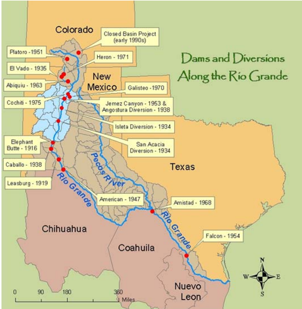
1 Figure A4.4. Dams and diversions along the Rio Grande. 27 2
