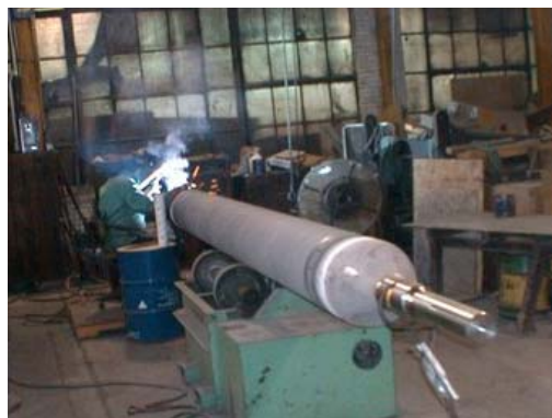
Advanced nickel aluminide materials used in transfer rolls of steel reheat furnaces reduce product defects and reprocessing requirements.
