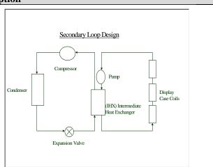
Secondary-Loop Refrigeration, where an extra pump and internal heat exchanger are added to the equipment used in a conventional design.
