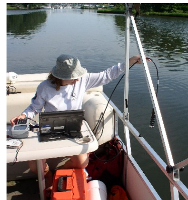
Maggie Payne using a YSI meter to measure water quality
