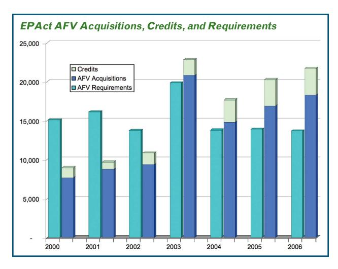
Vehicles. Flexible-fuel vehicles (FFV) that can run on E85 (85 percent ethanol, 15 percent gasoline) or gasoline were the AFVs of choice in FY 2004, FY 2005, and FY 2006. Of the 18,307 AFVs acquired in FY 2006, 18,067 were FFVs. The other AFVs acquired were compressed natural gas (CNG) vehicles. Similar trends were evident in FY 2004 and FY 2005.
