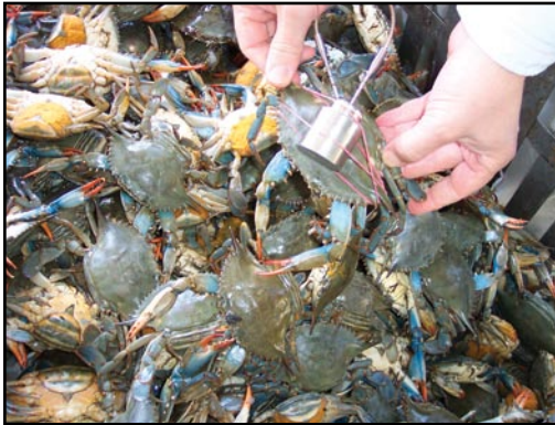
Fig. 3. A live blue crab with attached thermocouple is placed in steel basket before retorting begins.
