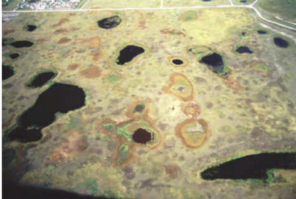
Figure 32. Aerial photo of the pothole area near Ninepipe, Montana. Note the high concentration of wetlands in the region and the diversity of pothole wetland types. Wetland density in this area is greater than 4 percent of the landscape. Distances should be measured between the project wetland and the five nearest neighboring wetlands, as illustrated in Figure 33
