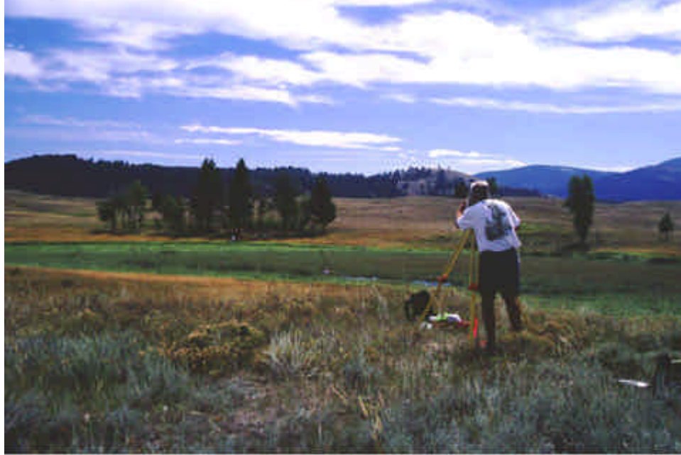
Figure 29. Proper placement of either a theodolite survey total station or an autolevel. Either of these instruments will greatly aid in rapid acquisition of needed geomorphic data
