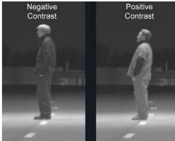
Figure 7. Photograph. Contrast of dark-clothed and light-clothed pedestrians.
