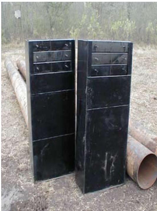
Figure 13-34 Pre-fabricated stoplog structures
