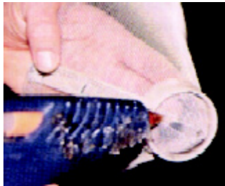
Figure 6E. Seal two layers of screening together.
