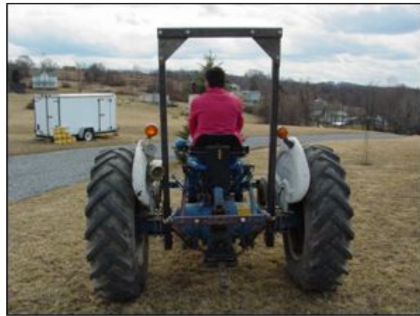
CROPS design for a Ford 4600 tractor.
