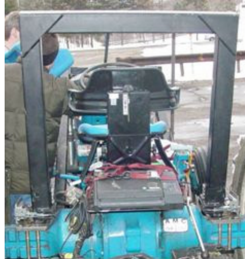
Third generation AutoROPS in a retracted position
