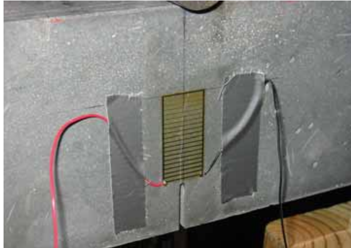
Figure 84. Photo. Resistance foil gage to monitor crack propagation.
