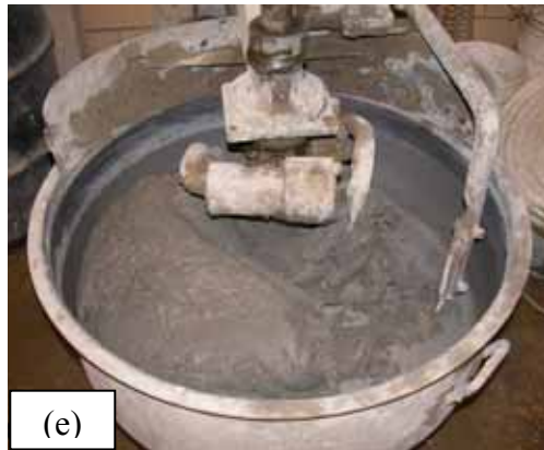
Figure 2. Photos. Mixing of UHPC. (a) Water addition. (b) HRWA addition. (c) Prepaste consistency. (d) Fiber addition. (e) Finished mix.
