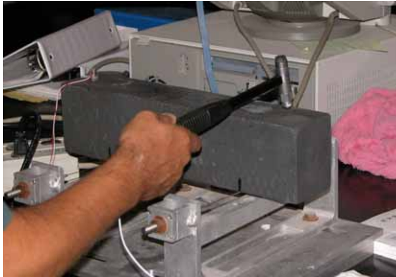
Figure 122. Photo. Resonant frequency testing of a freeze/thaw prism.
