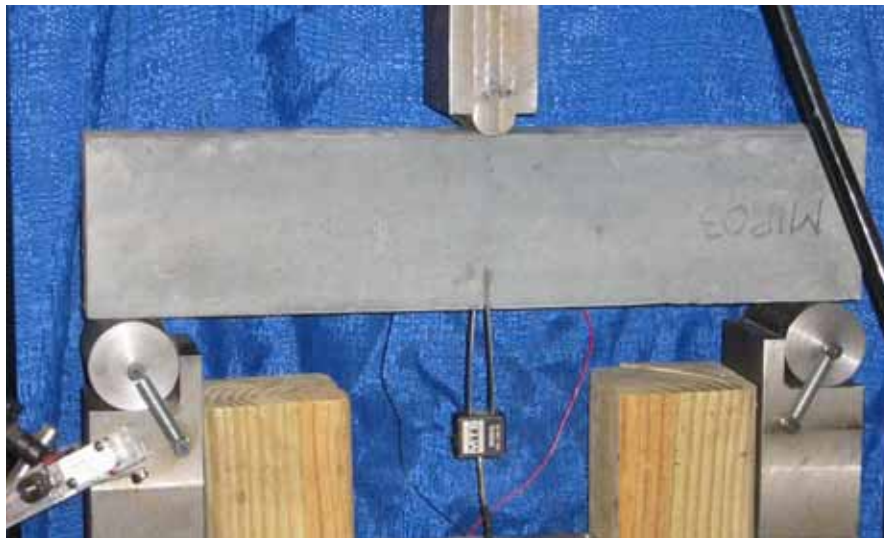
Figure 83. Photo. Test setup for 102- by 51-mm (4- by 2-inch) notched prisms loaded on a 406-mm (16-inch) span.
