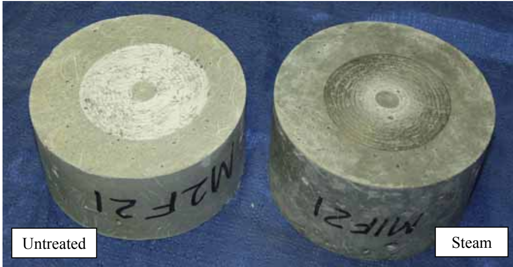
Figure 118. Photo. Steel cast surface untreated and steam-treated abrasion specimens after 8 and 10 minutes of abrading, respectively.
