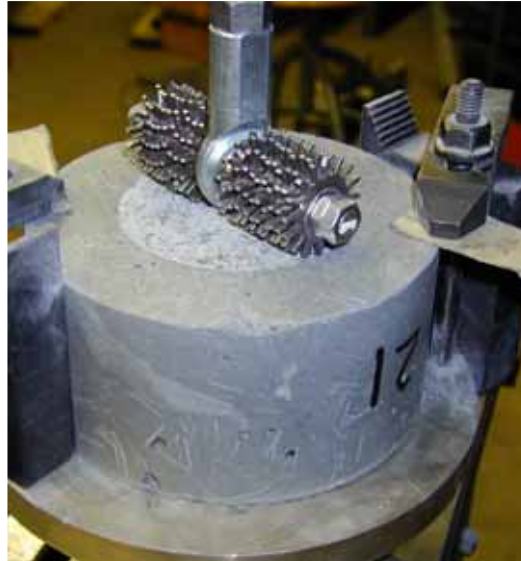
Figure 117. Photo. ASTM C944 abrasion test setup.
