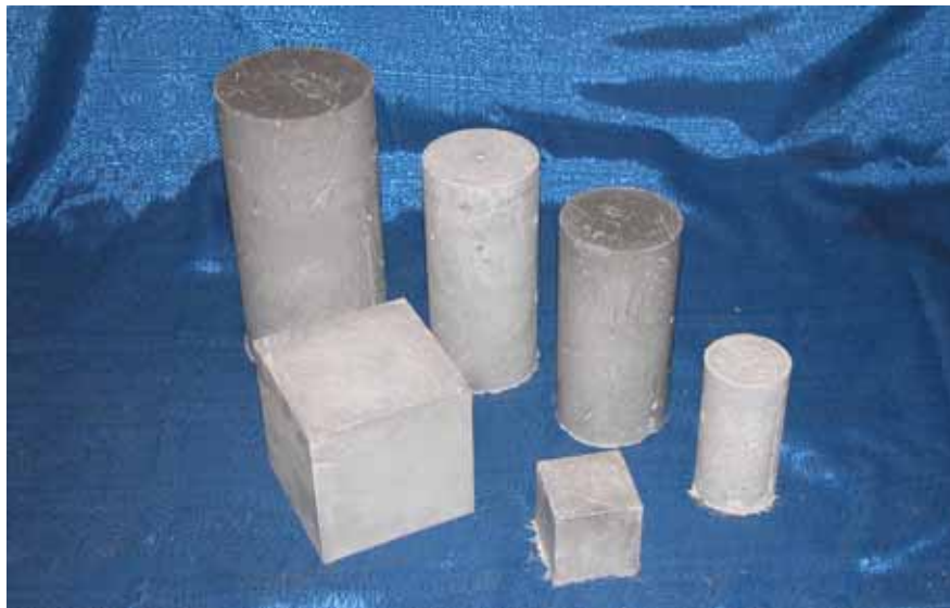
Figure 23. Photo. Compression cubes and cylinders including (clockwise from upper left) 102-mm (4-inch), 76-mm (3-inch) overlength, 76-mm (3-inch), and 51-mm (2-inch) diameter cylinders and 51-mm (2-inch) and 100-mm (4-inch) cubes.
