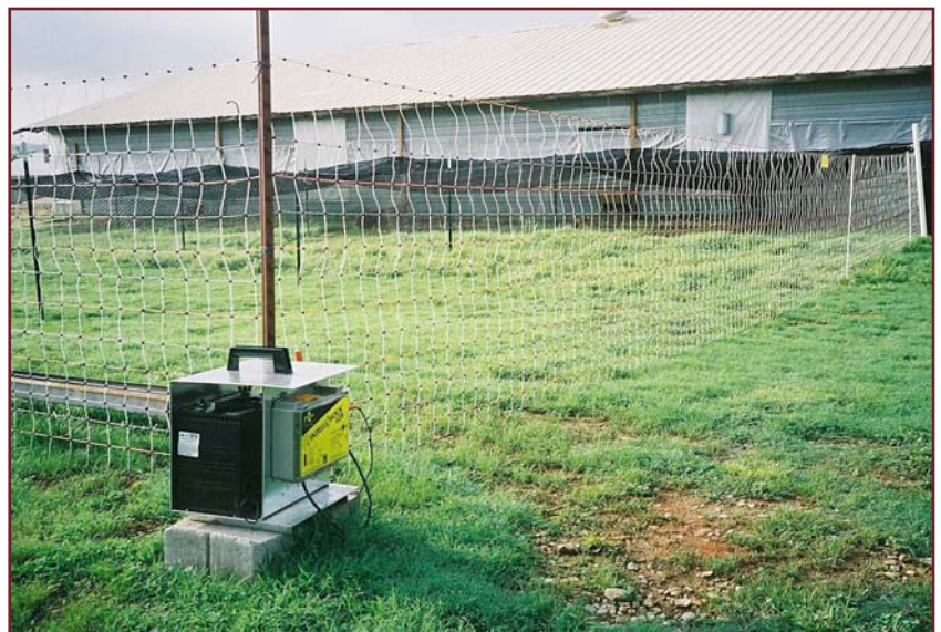
Electronet fence to protect birds from predators. Photo by Anne Fanatico, NCAT.
