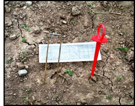
Metal wire staple left. Plastic staple right. Used to secure covering material.
