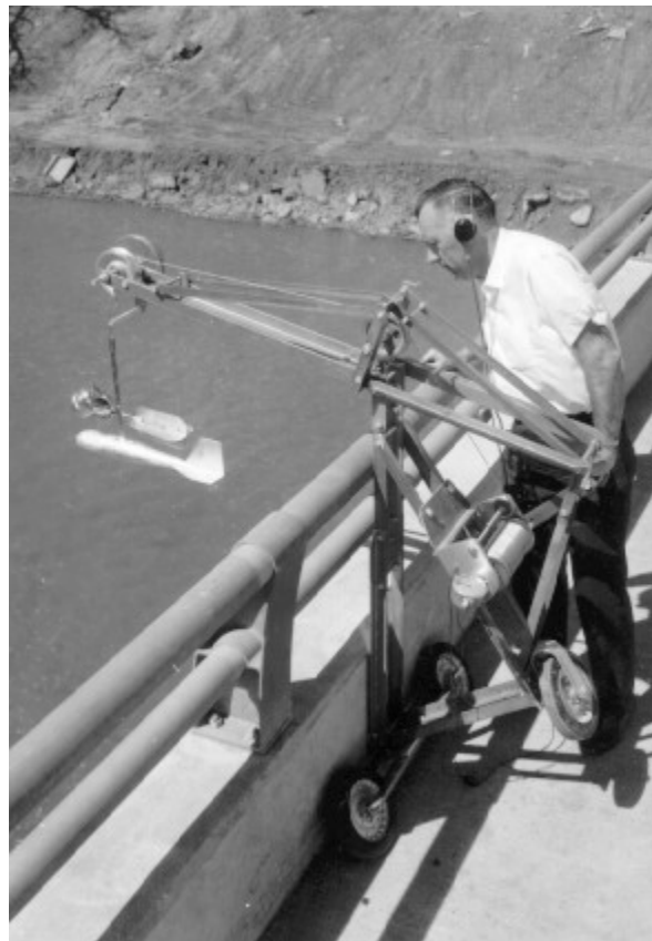
Figure 10-4 -- Type A crane and current-meter assembly in position on bridge.
