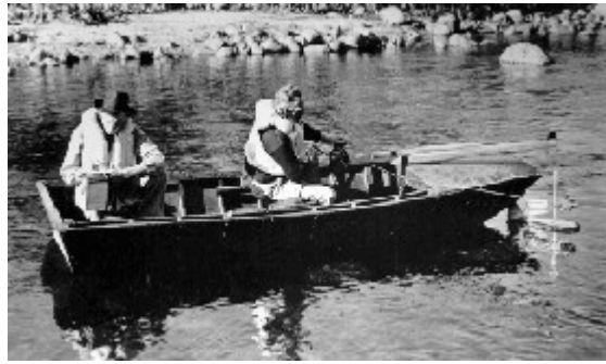
Figure 10-5 -- Making a current-meter measurement from a boat.
