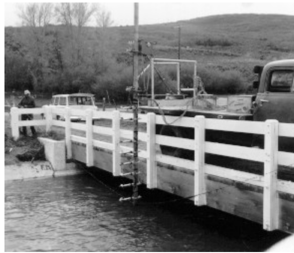
Figure 10-14b -- Truck-mounted assembly of eight propeller-type current meters and signal recording equipment used on Gateway Canal, Weber Basin Project, Utah.
