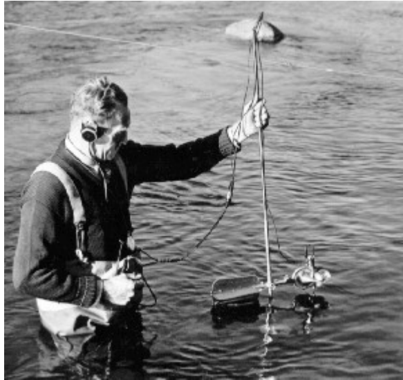
Figure 10-2 -- Equipment for making wading measurements with a current meter. Note tag line for marking stations.
