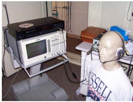
Photo 1. Test setup using KEMAR and SR785 analyzer
