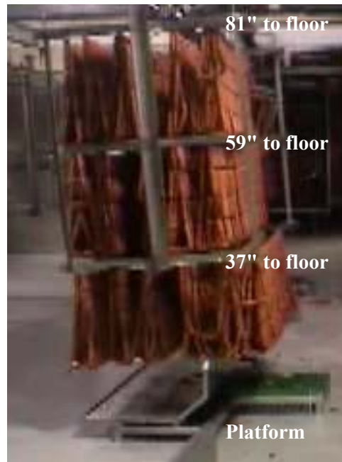
Photo 1. Fully loaded frank rack in the cooked production area with measured height dimensions.
