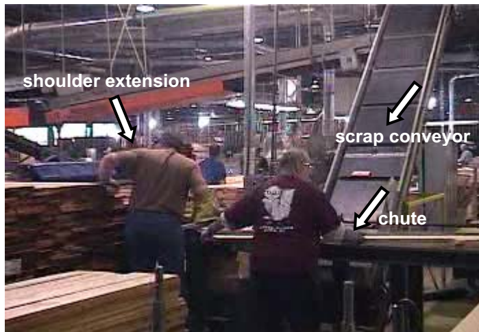
Photo 1. Stack height of wood is high, requiring full shoulder extension.
