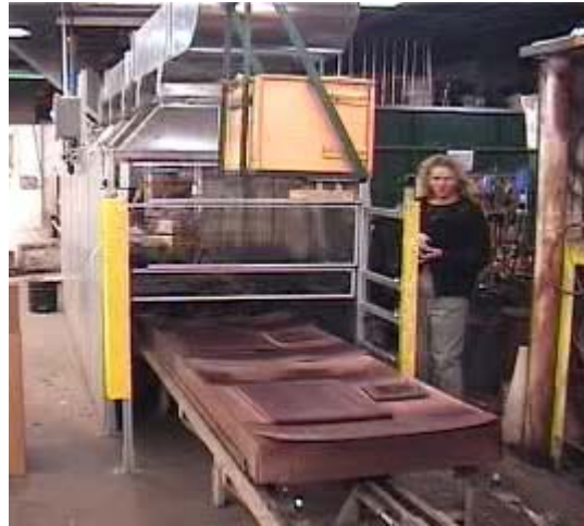
Photo 11. Low conveyor height placing workers at risk for low back pain.
