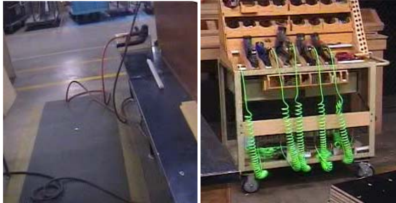
Photo 12. Loose hoses pose a tripping hazard (left); coiled hoses eliminate the trip hazard (right).
