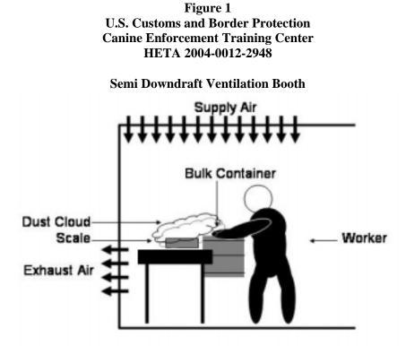
Filtered air enters from the ceiling of the booth, collects dust as it flows past the worker, and exhausts out the back of the booth through grates (side view).
