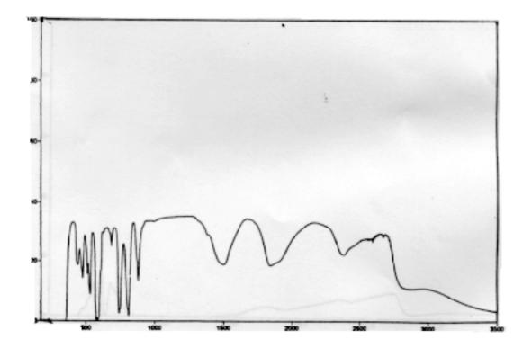
Transmittance / Nanometers Protective cycwcar having moderate UV, VIS, Blue, and IR transmittance
