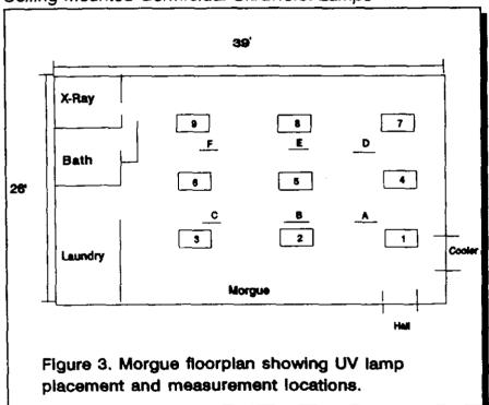
Ultraviolet (UV) radiation measurements were made at several locations in the moraue where the ceilingmounted GUV lamps are located (see Figure 3 left). GUV lamp placement is shown at locations A through F. Locations 1 through 9 represent sampling locations below fluorescent light fixtures. All lamps were in operation at the time the measurements were made, but bulb "C" was flickering. Measurements were made at a distance of 4 inches below the center of each lamp, at
