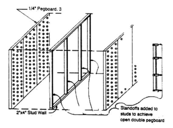
Figure 2 Construction Detail, Double Open Pegboard Inlet Using Standoffs Added to Existing Studs U.S. Park Police Firing Range Washington, D.C. April 24 and 25, 1991 HETA 91-124
