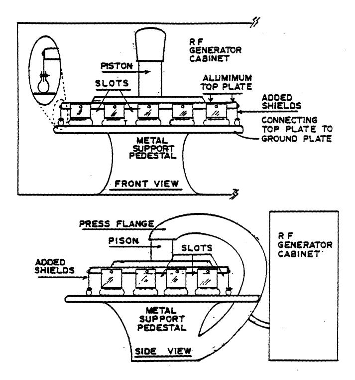
FIGURE 1. Phosphor-bronze spring shielding
