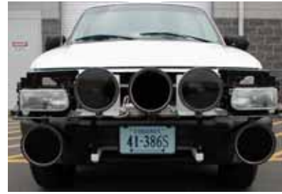
Figure 3. Photo. Headlamp setup on white SUV with five UV-A and HLB.
