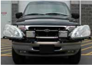
Figure 2. Photo. Headlamp setup on black SUV with hybrid UV-A and HID.
