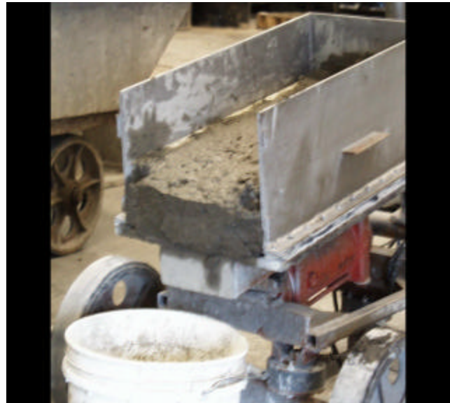
b. Concrete remains in the chute when the gate is removed.
