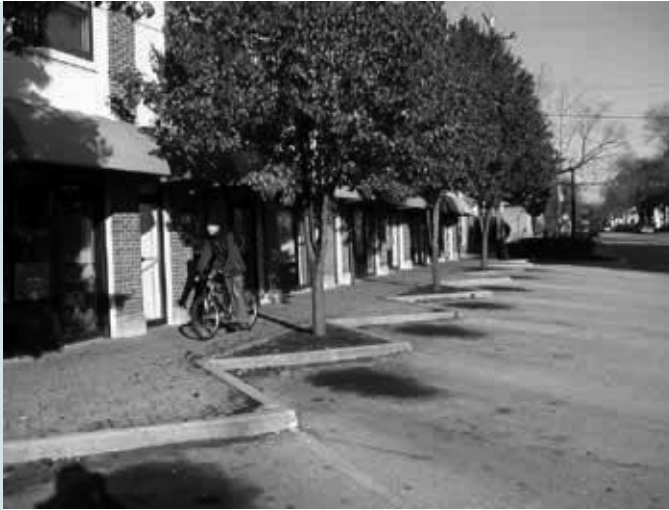
On-street parking can be coupled with tree wells in a downtown setting.
