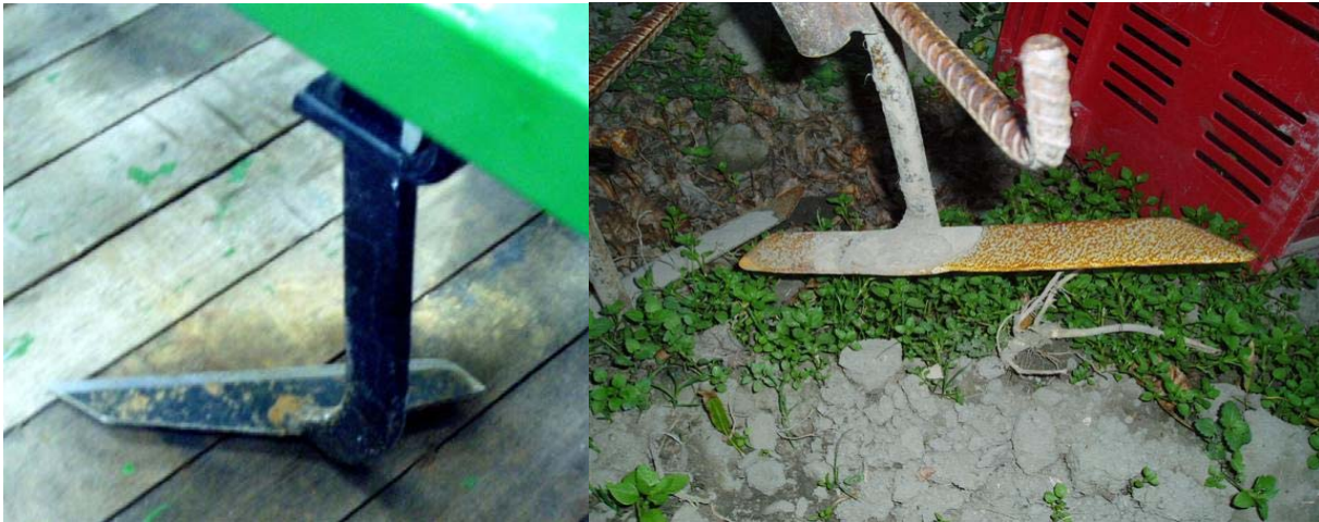
Figure 8. T hoe with the leg attached to the middle of the rear edge of the blade
