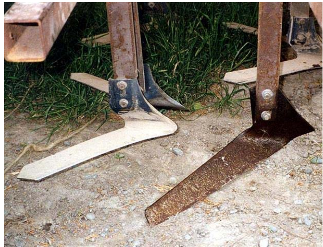
Figure 7. Poorer designs of hoe blades
