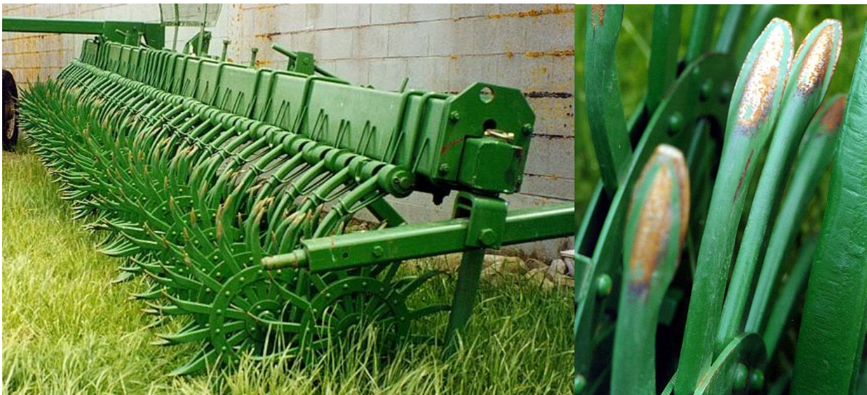
Figure 5. Spoon weeder / rotary hoe with close-up of spoon tips
