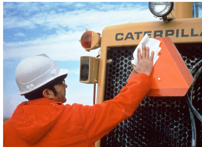
In addition to routine machine maintenance, it is very important to keep all warning devices clean and visible.
