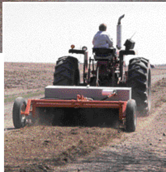
A commercially manufactured pulverizer.
