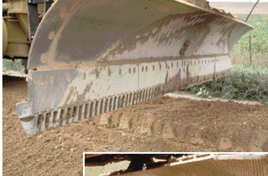
Examples of different types of replaceable bits for cutting edges.
