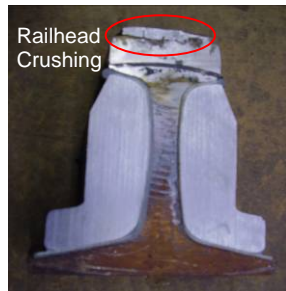
Figure 3a. Railhead Crushing, Prototype Removed after 300 MGT.
