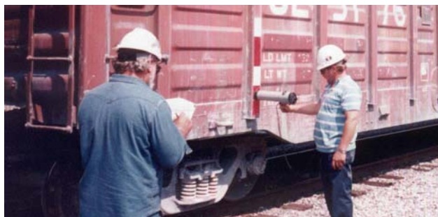
Figure 1. Mounting of Retroreflective Materials on a Box Car
