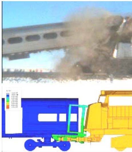
Figure 8. Conventional Train-to-Train Test Result and CEM Train-to-Train Test Prediction
