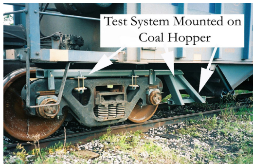
Figure 5. Field System on a coal hopper.
