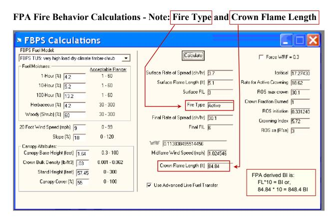
The preceding calculations can be made using Personal Computer Historic Analysis (PCHA) Version 1.3.0, Patch 1j. Calculation module is found under the Utilities tab, FBPS Calculations.
